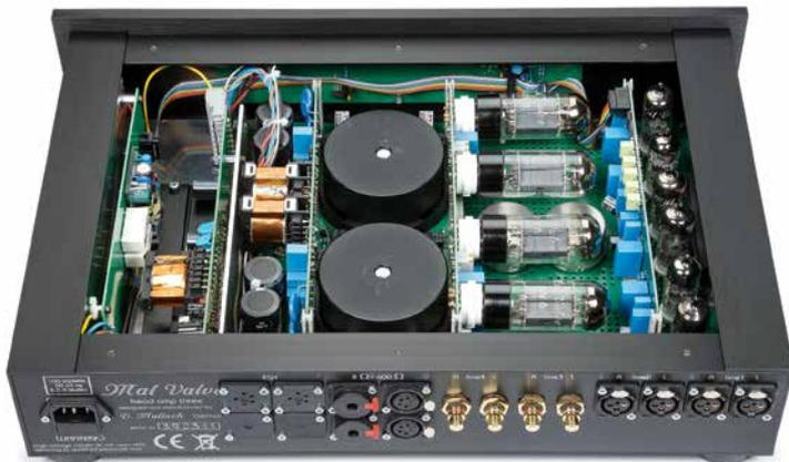
**The interior of the Mal Valve amp is constructed in a modular and extremely clean way. The power tubes deliver twelve watts per channel.**
